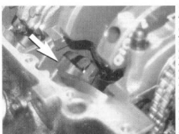
The 403 Olds is easily identified by its "windowed" main webs. (arrow) Most 403s had them, and they are sufficient to support a decent street engine. Taking advantage of the other design elements of the 403 will more than make up for the lack of material here. If spotting the main webs is too difficult, maybe the big "403" cast into the block will make it easier to identify.
