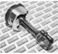
The factory connecting rods are fine for the 403 once they have been through standard prepping and resizing procedures. Note the polished beams and upgraded bolts, along with time-honored lightening and balancing tweaks that have become standard on all performance engines.
