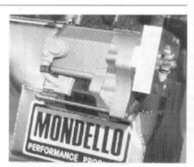
With our oil pan in place, Joe turned us on to this cool mini starter he recently began selling. Considering the fun any Olds owner has with header routing, we think one of these high-torque mini starters would be a good move. The small size makes working around the pipes easier, and it has more torque than the factory units.
