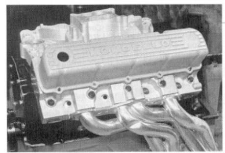
Head choices for the 403 range from the factory smog heads, to the decent 350 heads, to these killer Edelbrock aluminum castings. We think 403s weigh plenty already, and addition of these lightweight and efficient heads is the only way to fly.
