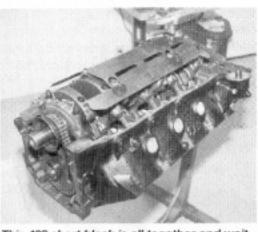
This 403 short block is all together and waiting for an oil pan. Things to note here include the windage tray, clearanced pump, and custom oil pickup. If you think oil control isn't a big deal in the Olds, you'd be wrong. What you can't see is the ported oil passages, restrictors, and improved drainback mods that Joe has found to be essential in keeping Rocket motors alive.
