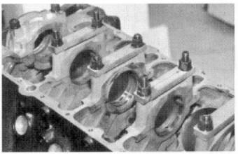
Strapping the main caps (as shown here on a 455) is an effective way to stabilize the mainline. Joe recommends this for all high-performance Oldsmobiles, but especially the mainline-challenged 403.
