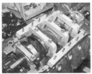
If you really want to get serious, Mondello sells this billet cradle for the bottom end. By spreading the load over such a wide area, the main bearings are fully supported and can handle the extra twists produced by high cylinder pressures and sky high rpm.
