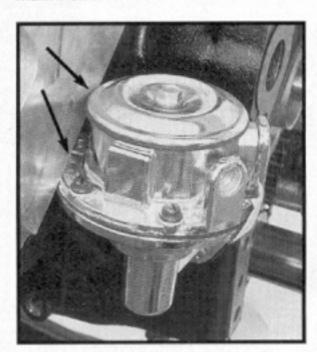
Edelbrock heads won't clear a smallblock Olds mechanical fuel pump (arrow). Don't try to clearance the head—you'll hit water. Run an electric fuel pump instead.
