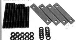
Mondello's main stud and strap kit (PN MS ST942) has provisions for the company's windage tray. The chromoly straps and ARP studs increase bottom-end rigidity and strength for big power levels.
