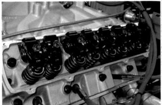
Once the engine was assembled, Mondello measured for pushrod length, then sent its measurements to Comp Cams, which quickly built and shipped a set of high-quality 4130 pushrods out the door. With lift numbers this high, valvetrain-component quality becomes critical. High spring pressures can bend inferior components, wear down poor-quality cam lobes, and just plain blow stuff up. We're more than confident in the quality of our Comp Cams pieces.
