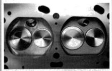
Mondello installed its PN SK700-700 valve springs for use with our solid roller cam. The springs were set to 250 pounds on the seat at 1.750-inch height. Also, Mondello's Posiflow 2.075-inch intake and 1.685-inch exhaust valves went in as part of its CNC valve job. The Mondello valves are swirl-polished, back-cut, and feature other proprietary tricks for improved flow. The combustion chambers were polished and slightly reshaped and smoothed (*left*).
