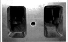
The intake and exhaust ports are also treated to some CNC cutting as part of Mondello's valve job (*right*) to improve the flow numbers by 35 cfm as compared with out-of-the-box heads. The new port window matches the wide mouth of Mondello's Posi Flow intake gaskets.
