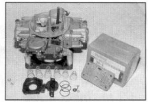
Holley carbs can be improved without radical modification. This Holley 3310 750 cfm four-barrel is shown with Moroso clear sight plugs, vacuum secondary quick-change kit, vacuum secondary springs and rear metering block kit. These parts, as well as pump cams, squirters and jets, are all available from Holley and specialists like the Carburetor Shop in Rancho Cucamonga, CA.
